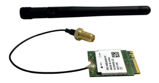
Our combined WiFi/Bluetooth module is for use with the MBS line of Mimo displays with BrightSign Built-In. This module enables the display with BrightSign Built-In to network using WiFi and operate BrightBeacon via Bluetooth.
