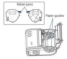
3. Align the two tabs on the paper guide with the slots in the bottom of the roll paper holder.
