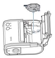
4. Firmly insert the metal part of the paper guide into the slot at the front of the roll paper holder.
