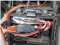
Figure 2 – Example of QuadSteer installed with receiver in an Axial
