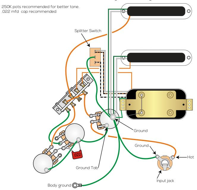
To use a Push/Pull pot, simply treat one side of the six lugs on the Push/Pull pot as the three lugs of the Mini-Toggle switch in the diagram above.
