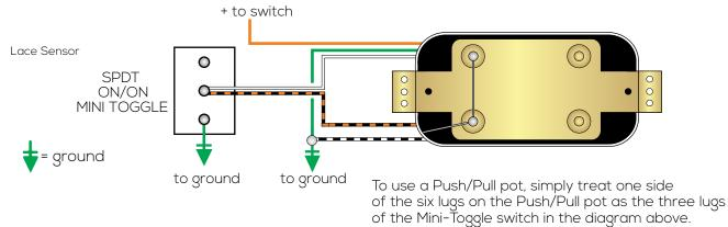
The Lace Sensor Dually can be wired for "Dually" mode: front coil/both coils/rear coil for 3 tones in one. Use SPDT on/off/on mini toggle switch. This also works for all Lace Sensor Humbuckers (excluding Alumitones)
