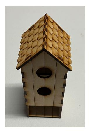
5. Then glue both the roof plates on, the slots will align and interconnect.
