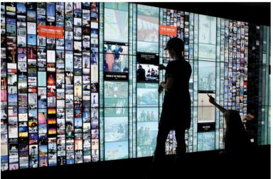
Planar's bundled solution in use at the observation deck at the Space Needle in Seattle, WA. Called the Sky Pad, the 135-square foot solution consists of 15 Clarity Matrix LCD Video Wall displays in a three-by-five configuration.
