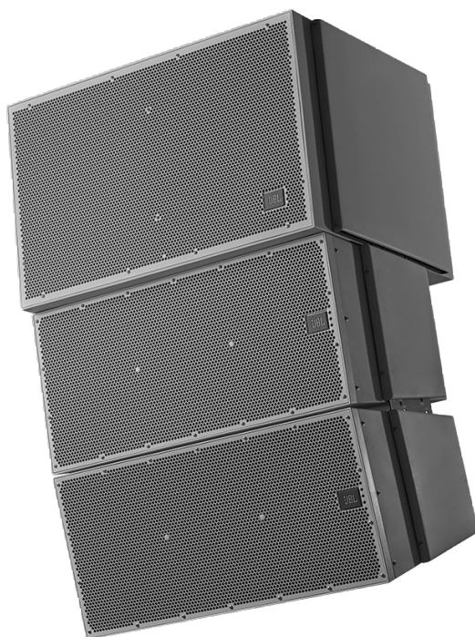
A member of JBL Professional's VLA Compact Series, the VLA-C265 is a two-way full-range loudspeaker with an outdoor IP55-rated enclosure for protection from dust and water. The high-frequency section is horn-loaded for maximum sensitivity and optimum pattern control. It offers three D2415 drivers featuring 1.5-inch diameter annular diaphragms, 1.5-inch voice coils, and neodymium motors.
