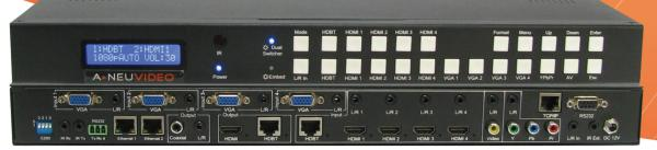
The ANI-11x2MFS is a multi-format video presentation scaler switch with audio. It features (11) Inputs of various video formats including HDMI, VGA, Component, Composite and HDBaseT™ with HDMI and HDBaseT™ outputs. Video can be scaled to various aspect ratios and resolutions from 640x480 up to 1920x1080@60Hz, and using by-pass supports up to 4K@30Hz.
