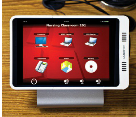
An iPad mini provides the control interface.
