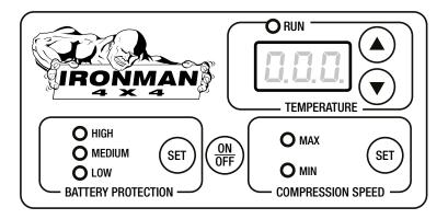
**Temperature Setting Range:** -18°C~10°C, -0.4°F~50°F **LED Display Range:** -20°C~40°C, -4°F~104°F
