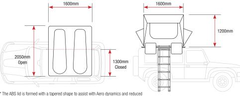
drag. When installed the tent will open to the right hand side of the vehicle.
