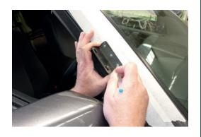
12. Apply silicone, insert mounting plugs and attach bracket using self tapping screw provided.
