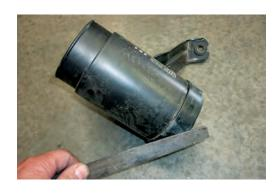
14. Apply silicone sealant to outside of rubber joiner in engine bay and attach rubber adaptor to it using hose clamp provided.
