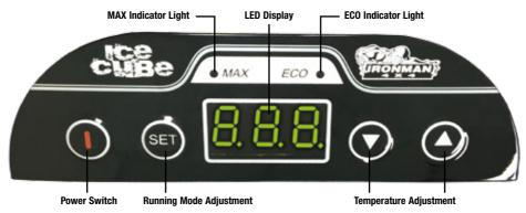
**Set Temperature Mode:** When the fridge is on, press and hold the SET button and momentarily press the ▲ UP button. The screen will display an 'F' for fahrenheit, or 'C' for celcius. Press the ▲ UP button to alternate between either mode. The screen display will flicker for 3 seconds, then auto-save your selection and automatically exit.
