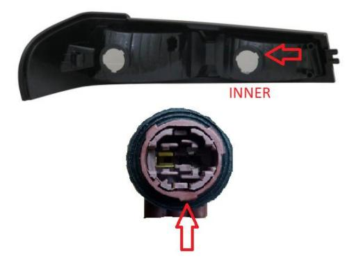
Once the sockets are inserted properly into the housings, reinstall the housings into the grille assembly. Reconnect the 3pin connector to the factory harness and try out the functionality of the harness.
