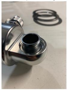
4.) Install the last snap rings into the bottom of the coilovers to retain the spherical bearings.
