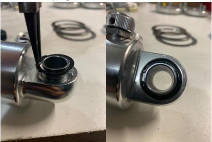
5.) Install the lower coilover perch locking rings on the coilover shocks with the flat face pointing downward. Thread the lock ring all the way to the bottom of the shock.
