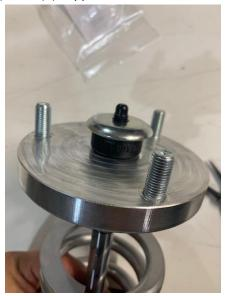
14.) Install upper mount nut. Viking provides two different nuts. Use the thicker one of the two.
