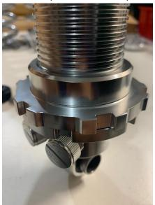
7.) Install the thrust bearing washers and thrust bearings onto the coilover perches. The order is: "Washer | Thrust Bearing | Washer"
