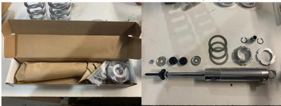
2.) Install (1) snap ring in the bottom of the coilovers.
