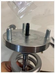
12.) Slide (1) upper mount bushing onto the shock shafts. Make sure to place the end of the bushing with the smaller piloting ring downward.
