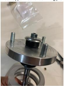
15.) Tighten the upper mount nut with a 14mm socket. An electric impact makes this step easier since the shock shaft will want to spin. Tighten the nut until there is ~.25" of threads showing.
