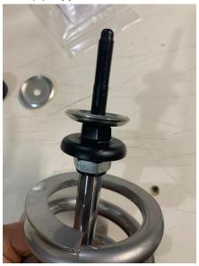
10.) Slide (1) upper mount bushing onto the shock shafts. Make sure to place the end of the bush with the smaller piloting ring upward.
