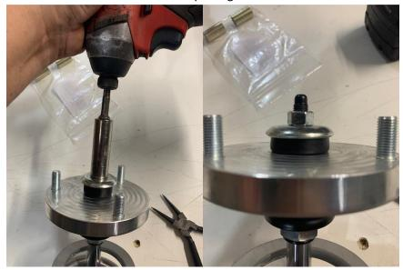
16.) Now turn the shock upside down so that the spring is centered and resting on the upper mount, and the thrust bearing assembly is centered and resting on the spring. While in this position, thread the perch and perch lock down until it contacts the spring.
