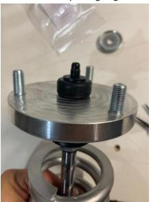
13.) Slide (1) cupped washer on the shock shafts with the cupped side facing downward.
