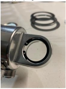
3.) Install lower spherical bearings in the coilovers.
