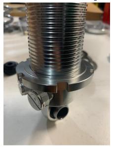
6.) Install the lower coilover perches on the coilover shocks with the flat face pointing downward. Thread the perches all the way to the bottom of the shock.
