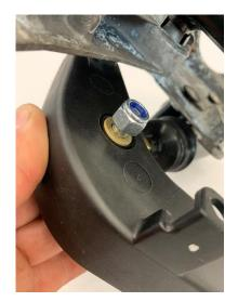
9. Tighten the nut <u>slightly!</u> Do not over tighten this nut. It only needs to be snugged up to the washers!
