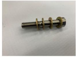
8. Insert the M8 bolt with the (4) 8mm washers through the hole in the left side of the clutch pedal, through the clutch master cylinder rod end, and out the right side of the clutch pedal. Place the other (4) 8mm washers and M8 nut on the bolt.
