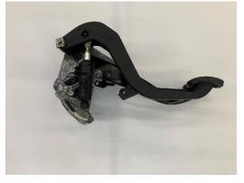
2. Remove the master cylinder pivot pin from the pedal
