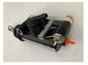
6. Using the (2) supplied M6 socket head screw, and the (2) M6 nut removed during step 3, attach the new master cylinder to the pedal assembly.
