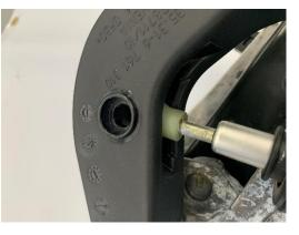
3. Remove the (2) M6 bolts from the master cylinder that hold the master cylinder to the pedal assembly mount. **Make sure to keep the (2) M6 nuts!**
