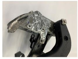
4. Using a file or sanding disc, sand down the raised portion of the forward most master cylinder mounting boss. **Do not sand too much!** You only want to remove the raised outer ring, and make the mounting boss flat.
