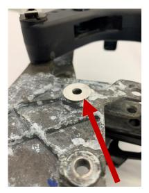
5. Install the spacer into the master cylinder mounting bracket.
