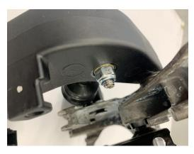
10. Put the new hose on the master cylinder, reinstall the pedal assembly, and bleed the system.
