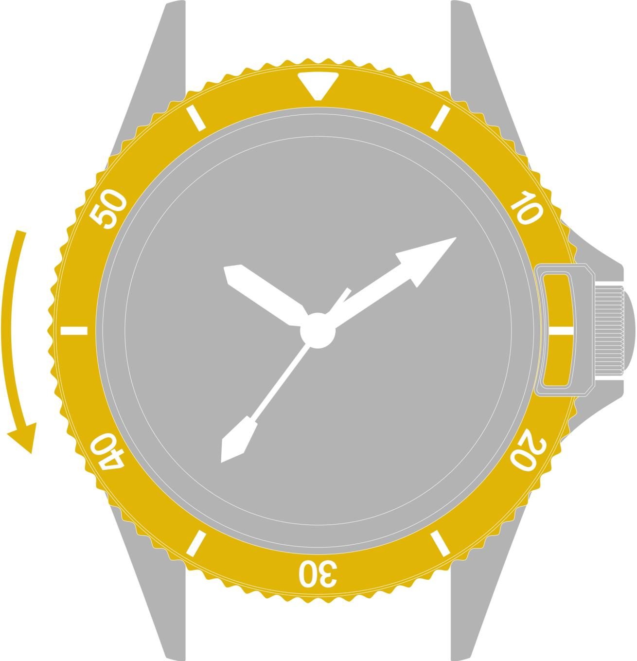
The unidirectional rotatable bezel allows precise measurement of dive times. For safety, the bezel rotates counter-clockwise only.
