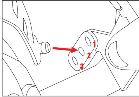
3. Then relocate the arm into 1 of 3 receivers. Repeat this process at all 4 adjustment points.
