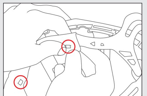
4. Hook the sweatband over the remaining tabs on the inside of the suspension.
