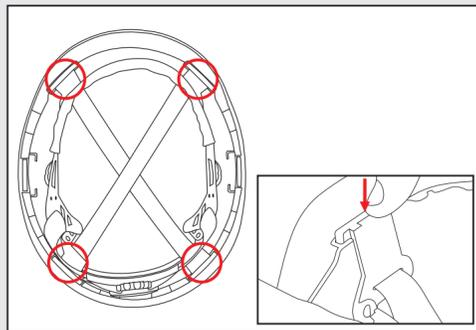
3. Place the new suspension inside the hard hat then click the first clip back down into position. Repeat the process for the 4 main clips.
