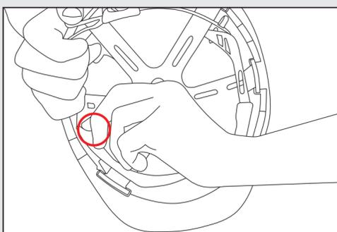
1. Remove the old sweatband from your EVO® safety hard hat by splitting at the weld at either corner and gently peeling the weld apart along the base of the old sweatband.
