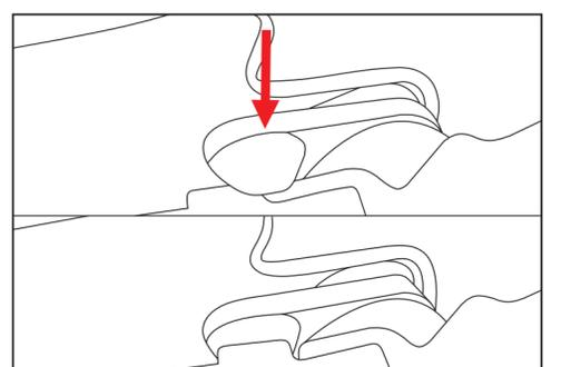
4. Push the spec down until the clips on the spec arm clip under the notches on the front webbing clips.
