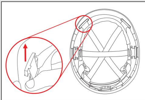
1. Remove the harness by placing your hand on the underside of the clip and pushing upwards and towards the back or front of the hard hat until it slides out of place.
