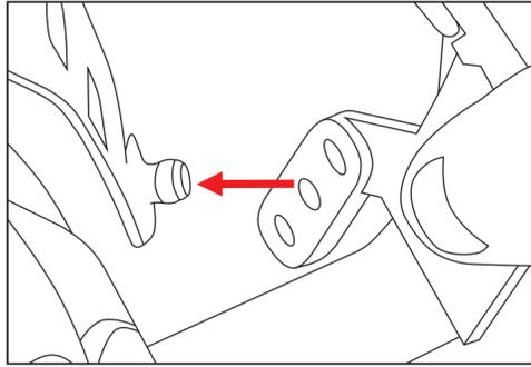
2. To adjust the height, un-pop the arm from the receiver (hold the hard hat and receiver firmly whilst doing so).
