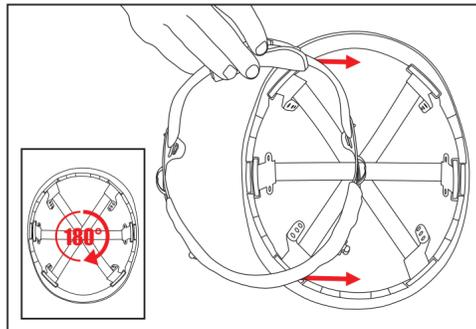
3. Now simply rotate the hard hat by 180° and place the suspension back inside.
