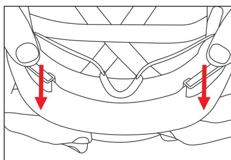
3. Once both pins are connected, slide the spec into the hard hat.
