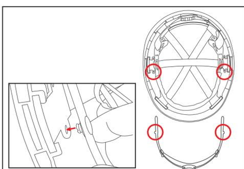
2. The pins on the spec arms go into the sockets closest to the front of the hard hat in the centre webbing clip.
