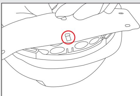
2. Place the holes from one side of the band over the tabs on the outside of the hard hat's suspension.
