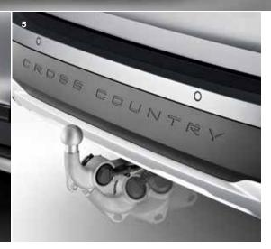
1. Protective steel grille. Load compartment divider. Dog gate. Load liner. 2. Load compartment mat, plastic. 3. Illuminated load scuff plate. 4. Mud flaps, front. 5. Semi-electrical foldable towbar.
