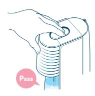
**FIRMLY PUSH** the carbonation button all the way down. **HOLD DOWN** the button for **1 SECOND**, and **RELEASE**
