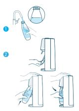
Note: when inserted correctly, there is a small gap between the bottom of the Carbonating Bottle and the base. Do not carbonate if the Carbonating Bottle is resting on the base, or water will splash out.
