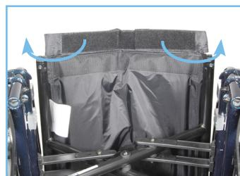
2. Pull outward on hook and loop fastener strips to free them from underside of seat.
