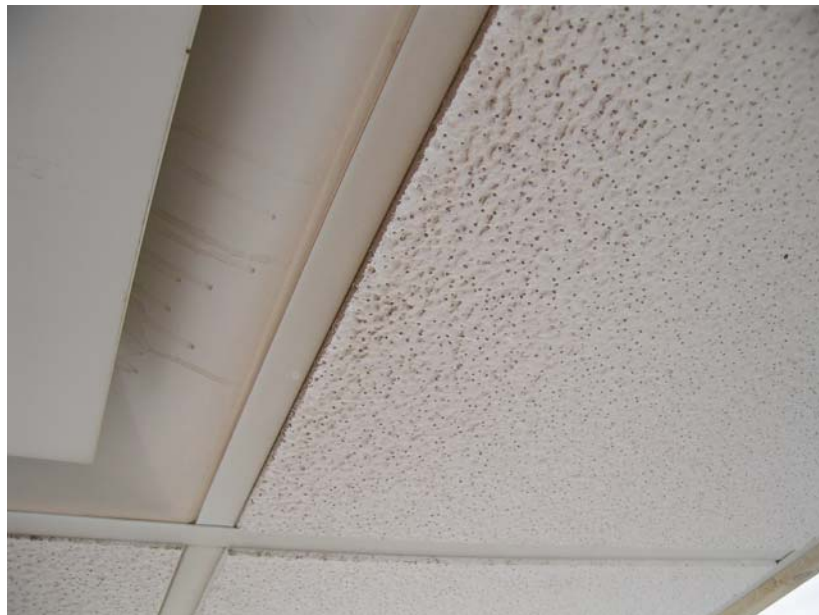
Figure 13: North tile after 202.5g of dispersed ball clay powder without a deflector
