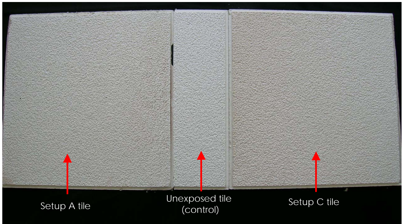
Figure 20: Comparison of Setups A and C to control tile
