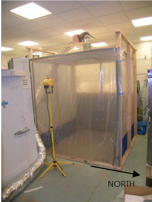
Figure 5: Test Setup: 6' X 6' simulated room with 7' suspended ceiling
