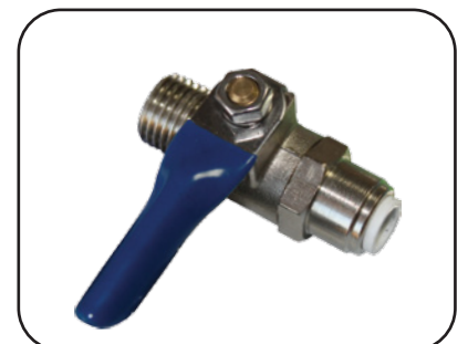
Metal Ball Valve "Closed" (Valve handle perpendicular to tubing)
