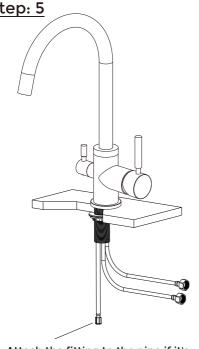
Attach the fitting to the pipe if it's not already attached
