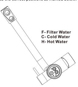
$\underline{Step: \ 1}$  Attach the lock bolt to the tap
