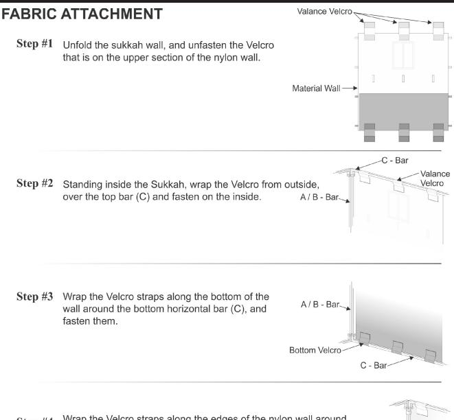
Step #4Wrap the Velcro straps along the edges of the nylon wall around<br/>the vertical corner/extension bars (A/B).
