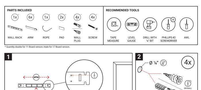
DETERMINE POSITION OF RACK AND MAKE A MARK THROUGH ALL FOUR HOLES. ENSURE RACK IS LEVEL. ACCOUNT SPACE FOR SECOND RACK FOR 11 BOARD VERSION.
