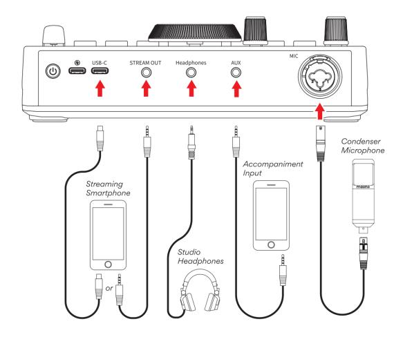
Connect the microphone to the audio interface using the XLR connector, making sure that the connection is tight and the connector is correct.
