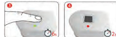
**Note:** The sensor is equipped with 360° Fingerprint Recognition Technology. Fingerprints can be scanned at any orientation as long as the correct part of the finger is presented to the sensor. After completing setup, ensure the accuracy of the profiles by testing out the scanner. If the readings are unreliable, follow instructions in part 7 and restart the setup process.
