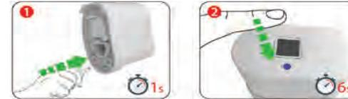
**Step 3:** Press any of your fingers (other than the enrolled Administrator's) onto the sensor and release, repeat this TEN TIMES (you will see the blue LED light each time)
