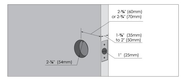
Deadbolt slot must align to the center of the door hole. Adjust as shown if needed.
