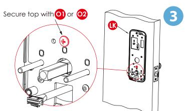
Pull the cable from the lock exterior through the rectangular hole underneath the positioning rods and spindle.
