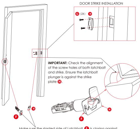
Make sure the slanted side of Latchbolt is closing against the slanted part of Strike Plate H before fixing it on to door frame.
