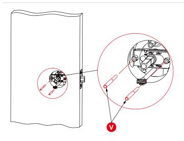
Insert Positioning Rods Vinto the holes to the left and right of the Spindle ©.
