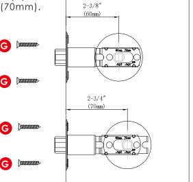
Facing the door exterior, install the lockset according to the opening direction of your door.
