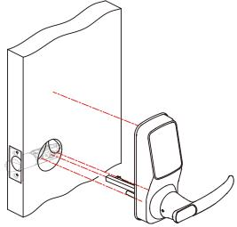
Install the exterior lock as shown to the left by aligning the lock straight and passing the cable and attached rods through the lockset.
