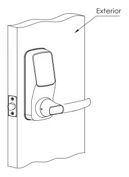
Align the lock straight and press hard (if you use the Adhesive tape in step 3.4) to secure the top of the lock.
