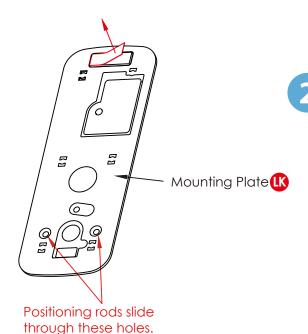
Interior Mounting Plate will go against the interior side of your door. Remove the paper layer off of the Adhesive Tape and align the positioning rods on the bottom of the plate to the corresponding left and right holes.
