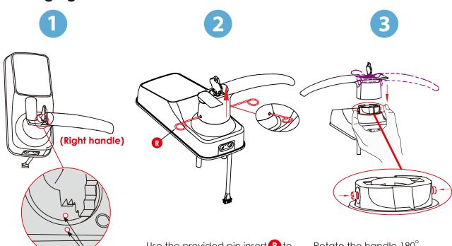
Insert key and rotate lock face so that the two white dots align as shown. Use the provided pin insert R to push the metal pin located at the 3 o'clock of the the base handle, then the other pin at 9 o'clock position. Remove the handle once the pins are compressed.
