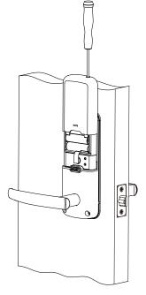
Insert 4 AA batteries into the lock by aligning the positive + and negative orientation markings on the batteries to the battery chamber.
