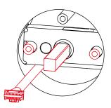
Pass the Spindle C through the center of the lockset, and the round rods through the sides in their respective holes. The cable should run underneath the lockset.
