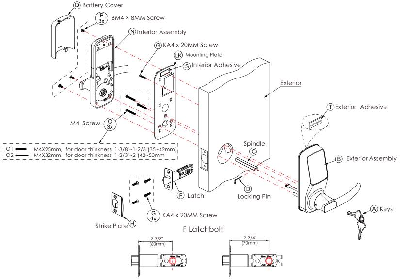
Measure distance between the center of the hole to the edge of door, adjust latch F to 2-3/8"(60mm) or 2-3/4"(70mm)
