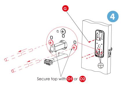
Remove the position rods V and replace them with screws Tighten clockwise until the mounting plate is secure.
