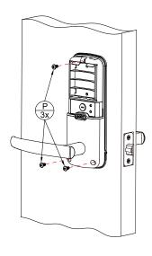
Once the lock interior is flush against the mounting plate, secure the lock to the plate by screwing clockwise using provided screws P.
