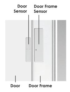
When you are installing the Door Sensor, make sure the arrows on the Door Sensor is placed next to the arrow from the Door Frame Sensor.
