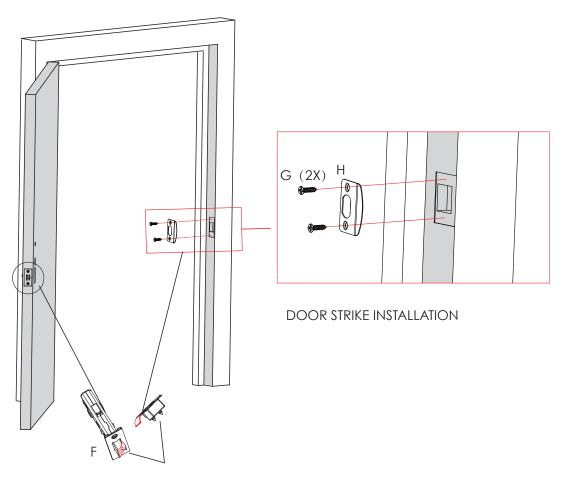
Make sure the slanted side of Latchbolt **(F1/F2)** is closing against the slanted part of Strike Plate **(H)** before fixing it on to door frame.
