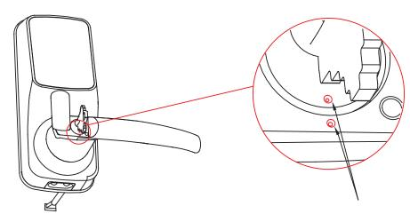
Insert the key and rotate to align the two white dots as shown in the picture.
