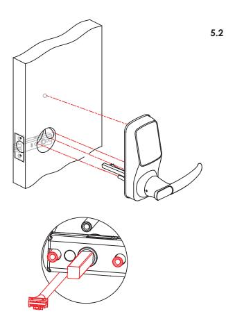
Install the exterior lock as shown to the left by aligning the lock straight and passing the cable and attached rods through the lockset.
