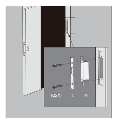
IMPORTANT: because doors and frames vary in design it may be necessary to make slight adjustments to your strike plate and/or dust box in order to ensure smooth hook operation. This is very important. If the hook is binding or catching in any way the lock will sound an alarm (rapid beeping) indicating it cannot close due to misalignment and/or excessive rubbing or binding.
