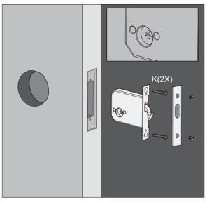
**4.** Attach the Face plate (V) back to the lockset (J). Secure face plate with screws W (2X).
