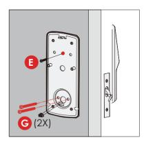
3: Insert and tighten by hand 2 © screws located on the left and right of the blade. Check alignment and tighten with screwdriver until mounting plate is securely placed on door.
