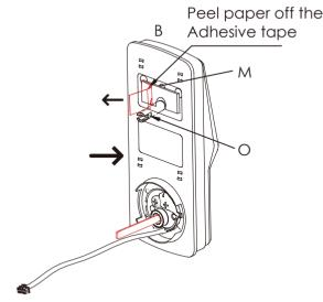
2: Before placing the exterior assembly on the door, make sure the torque blade is in vertical position and the hook is extended.
