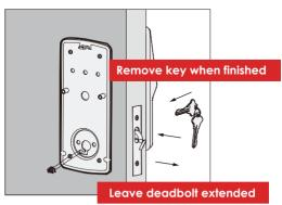
4: After securing the mounting plate, use the key to ensure hook locks and unlocks smoothly (no binding or rubbing). **IMPORTANT:** when finished, leave the hook extended and remove the key before proceeding to the next step.
