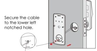
2: Place the mounting plate on the interior side of the door. Guide the cable to the opening ear on the side of mounting plate and make sure the torque blade is at the center of the mounting plate.
