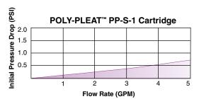
Data include cartridge and single-cartridge housing.
