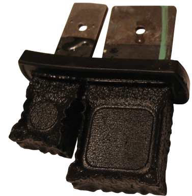
Chloramine damage on a valve disc used in a water treatment product.
