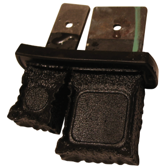
Chloramines damage on a valve disc used in water treatment product.
