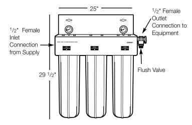
Mounting Depth: 15 <sup>1</sup>/<sub>8</sub>" Operating Weight: 90 lbs. Allow a minimum of 4" clearance under the filter to facilitate cartridge change.
