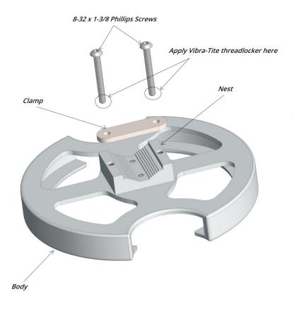
The String Caddy™ is designed to be clamped to your string trimmer's shaft.
