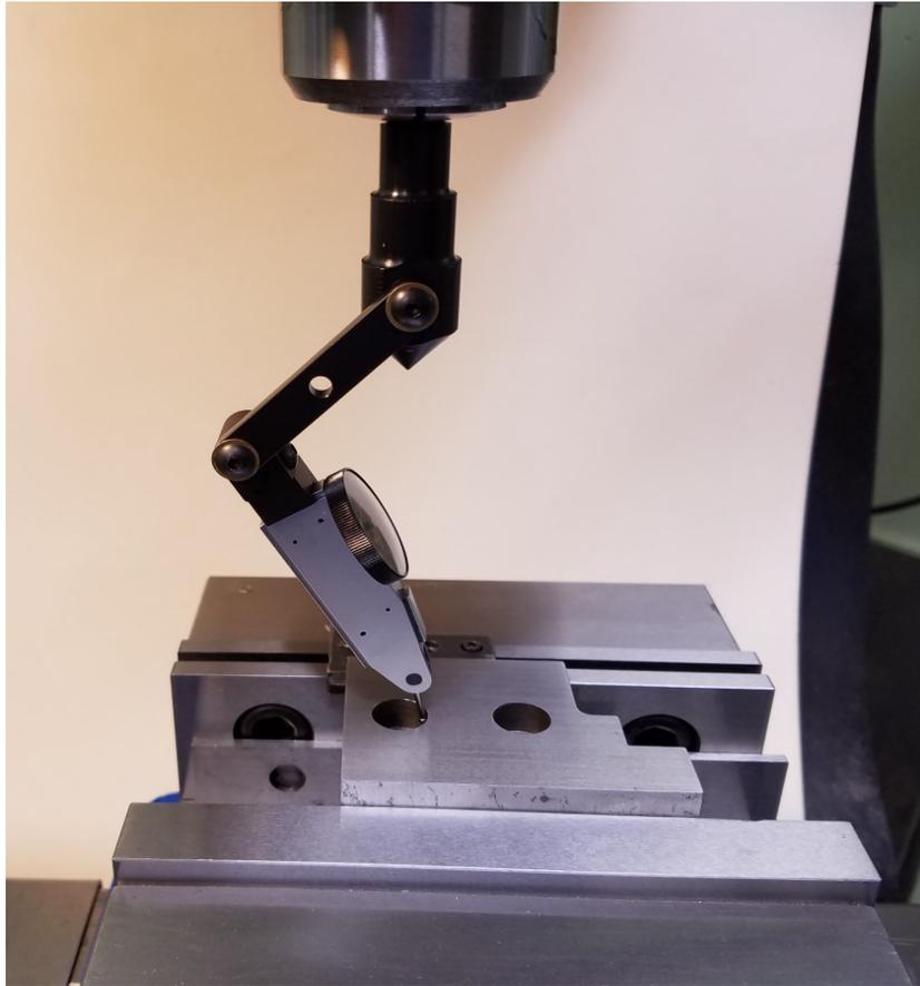
***The Inline Indicator Holder can speed up the process of finding the center of a hole or pin, because you shouldn't have to change the collet to fit the shank, and you can use the point to quickly find the rough center.***
