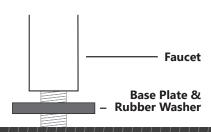
**7b**. Under the sink. install the Rubber Washer and the Tension Hand Screw over the threaded stem. Attach the Union Connector.
