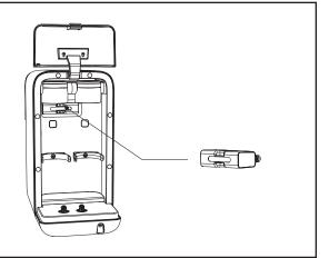
Reset and replace the water tank, fixing it tightly into place, and close the water tank cap.
