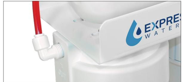
**4. Remove the Red Plug.** Secure the Red Tubing into the Male Elbow Fitting. Push hard enough on the tubing to make sure the Quick Connect has locked before moving on.
