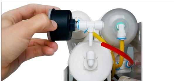
**1.** Put the end of the Pressure Gauge into one of the top arms of the Stem Tee. Then, put the Red Tubing into the opposite end as shown. Both will go about 5/8ths inch into the tee to secure.
