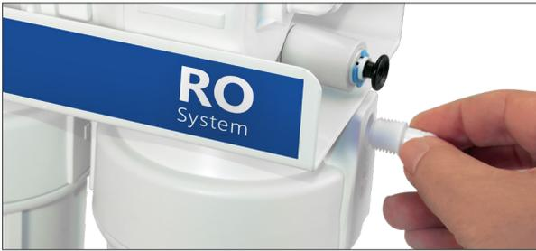
**1.** Screw a Male Elbow Fitting into the right-most Filter Housing (Sediment) marked "IN". Screw until tightened and the arm of the Elbow is facing downward.
