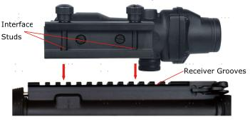
The 4X32 can be placed in any of the slots on top of the receiver to allow for eye relief adjustment. Once the ideal position has been determined, apply forward pressure on the optic and tighten the knobs firmly using finger pressure only. Then, add no more than another 1/4 turn utilizing a coin or a bladed screwdriver. This will ensure the mount will not loosen under recoil.
