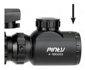
2. Adjust the reticle's brightness and color as needed using the illumination adjustment knob on the top of the eyepiece. Turning it towards you (clockwise) will first increase the brightness in the current color and then change to the next color, beginning at its lowest brightness. Turning it away (counterclockwise) will first decrease the brightness in the current color and then change to the next color, beginning at its highest brightness.
