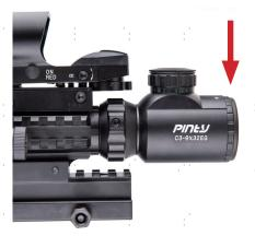
2. Adjust the reticle's brightness and color as needed using the illumination adjustment knob on the top of the eyepiece. Turning it towards you (clockwise) will first increase the brightness in the current color and then change to the next color, beginning at its lowest brightness. Turning it away (counterclockwise) will first decrease the brightness in the current color and then change to the next color, beginning at its highest brightness.
