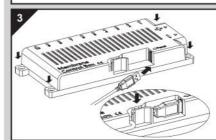
Install the Control Box properly with the included screws.
