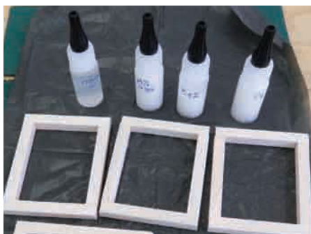
Development test panels for Deluxe Materials Tissue Paste experimental formulae. This looked at adhesive behavior.
