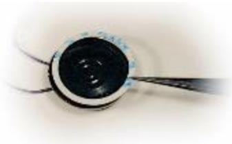
*Figure 10: SoundTraxx Speaker Gasket Installation*
