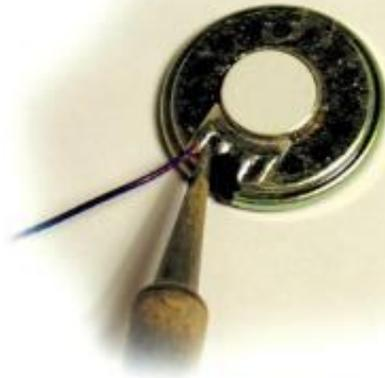
Figure 12: Soldering to Speaker Terminal Connections
